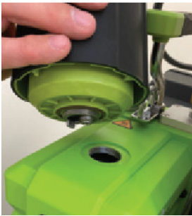
FIGURE 7: Demister removed, showing oil opening
